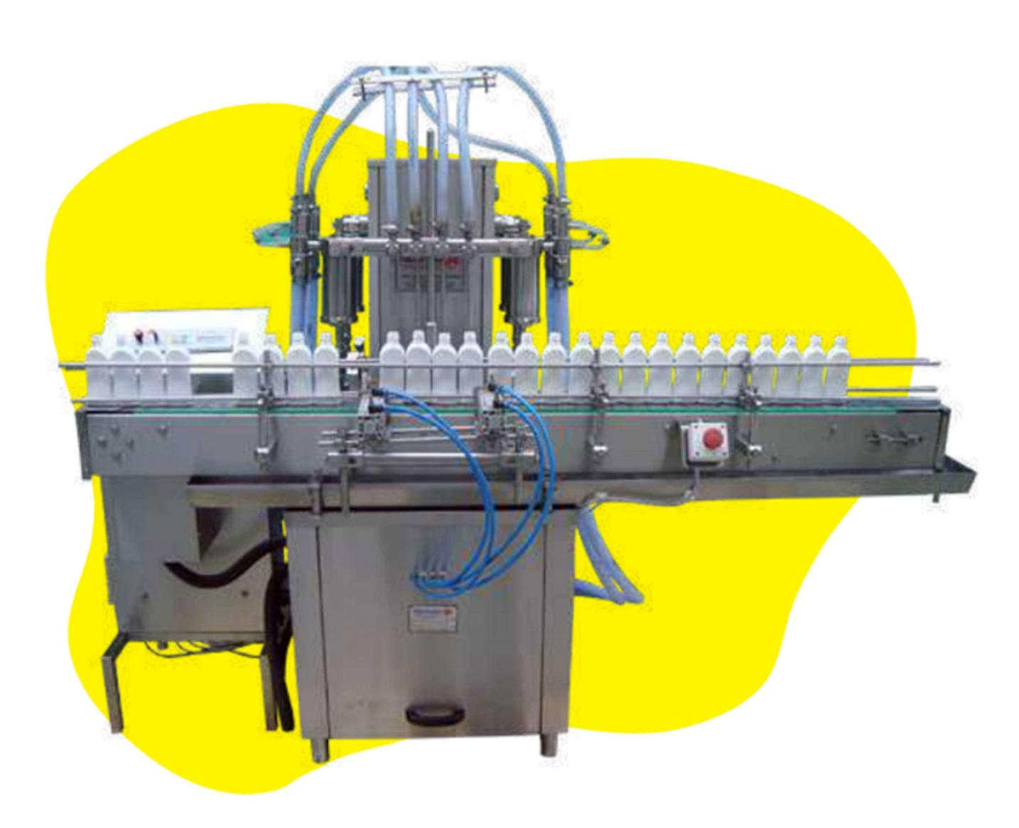
Our Automatic liquid filling equipment is of world-renowned quality with efficiency, precision, dependability, and flawless finishing, which can fill 40 bottles per minute. It supports industries like Chemicals, pharmaceuticals, cosmetics, food, and beverages. Advanced technology is included in an automatic liquid filling machine to enable accurate and consistent filling of liquids, from thin to very viscous materials like juice, ghee, oil, milk, syrup, honey, and more liquid products.
